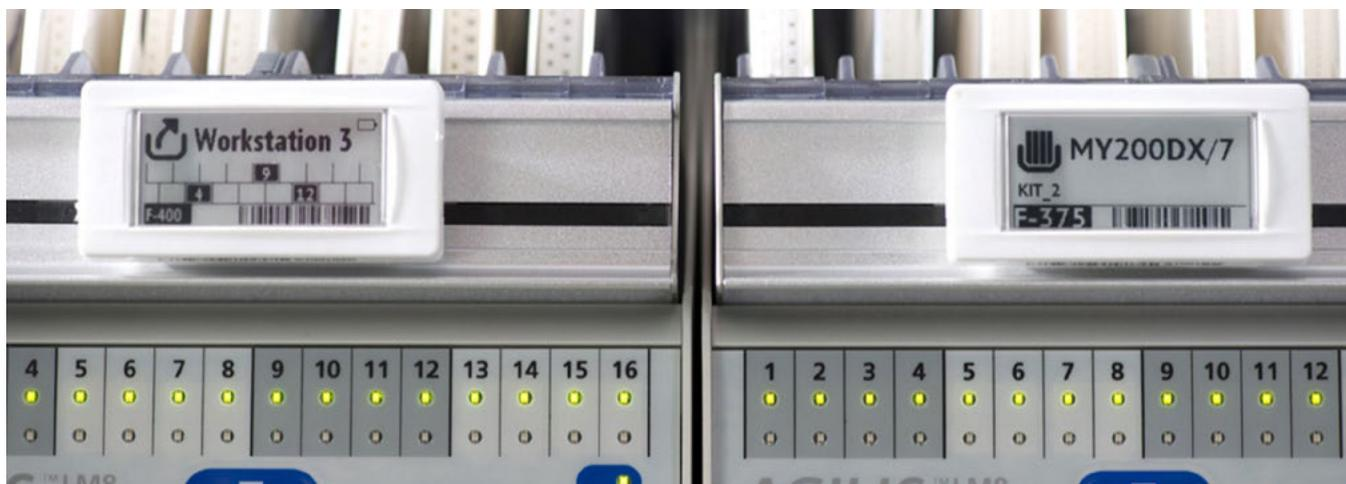
Figure 1: The challenge for many is to keep track of where they have their materials and to have an official material flow in the factory. Mycronic's material handling system can track the quantity and current location of each individual reel, stick or tray.
