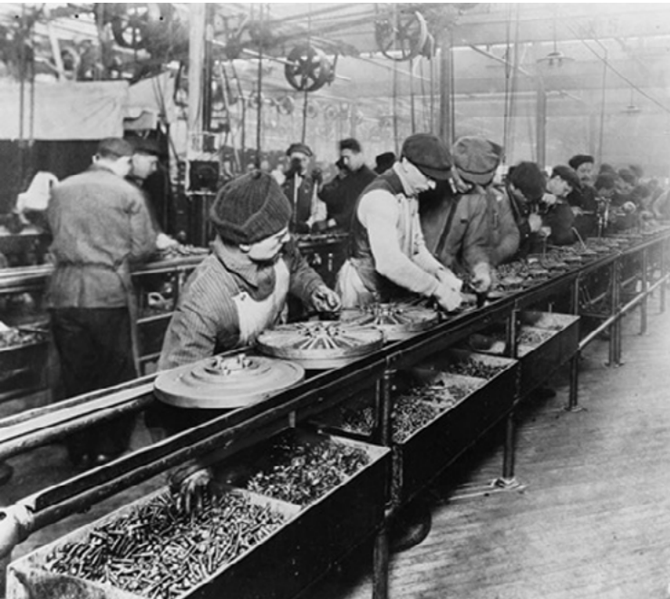
Figure 3: Magnetos and flywheels being assembled on the first moving assembly line in 1913, Highland Park, Michigan. (Courtesy US Department of the Interior)
