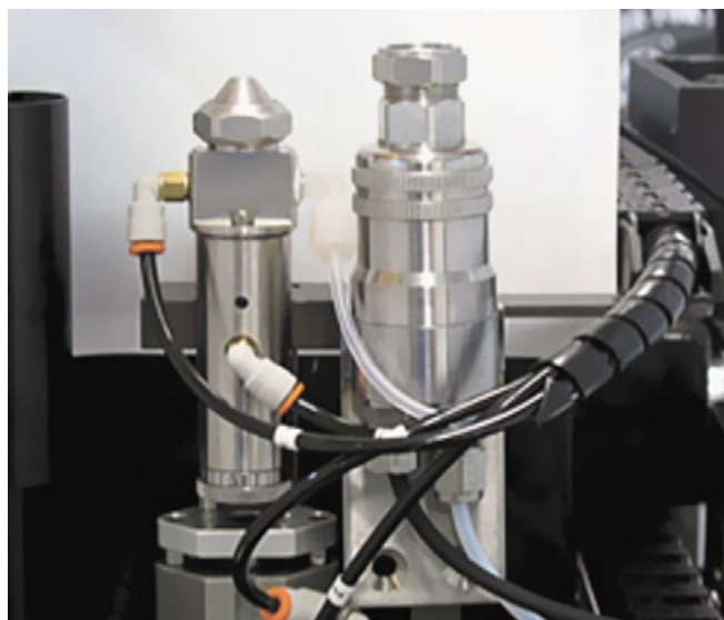
Figure 1: Drop-jet fluxer nozzle (right) and standard nozzle (left).
