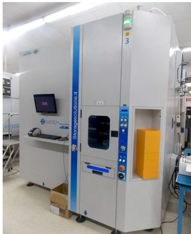
ISM2000 automatic store for SMTs and THTs in use at Whizz Systems.
