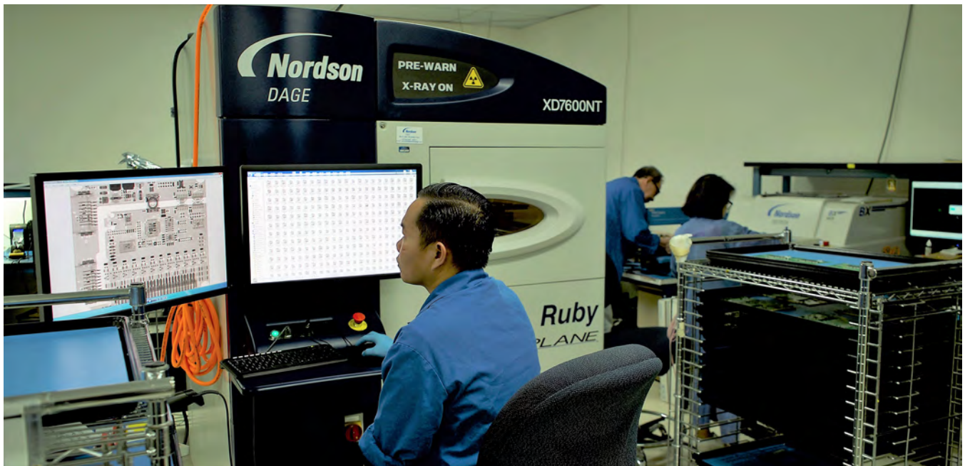
Whizz Systems technician using X-ray inspection equipment.
