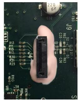
Figure 2: Peelable mask for conformal coating.
