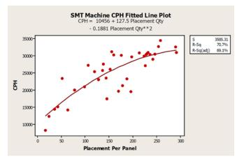
Figure 3: Fitted line plot of SMT machine CPH predicted by placements per panel for less than 300 placements per panel.
