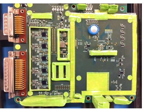
Figure 1: Pre-cut tape shapes for masking.
