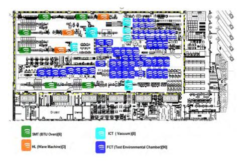
Figure 8: IIoT control vs. line layout.
