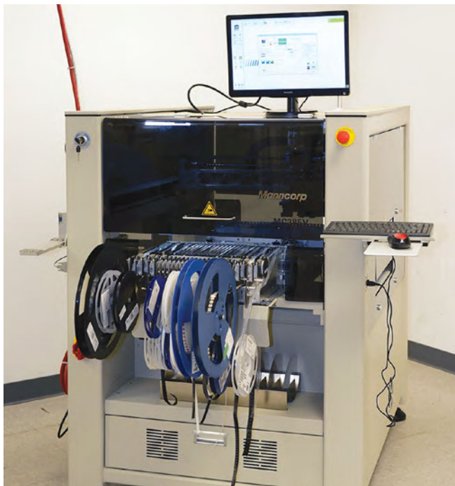
Figure 6: Sensorcon's new production line includes the 2-head MC-385 pick and place system, the same model Verbos uses to build his synthesizer modules. At 8000 CPH and $65K it ranks as one of Manncorp's most popular systems.
