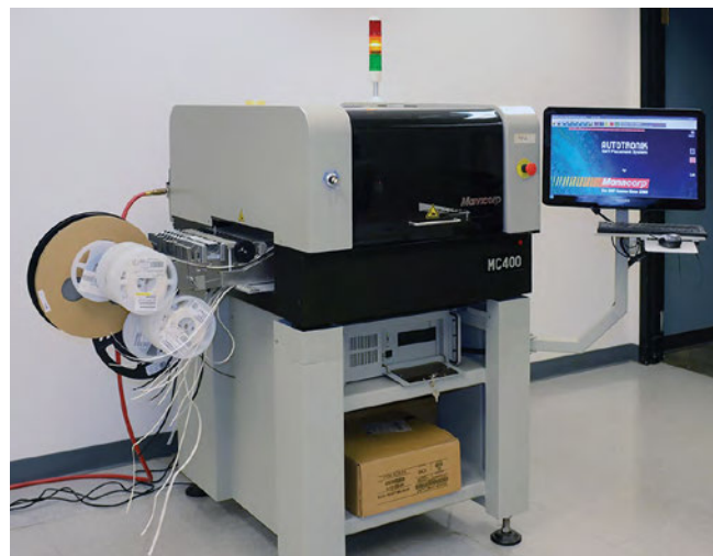
Figure 5: With the addition of their second Manncorp SMT line, Sensorcon's 3000 CPH MC-400 pick and place will now be used for new product development. Its feeders are interchangeable with their new MC-385.
