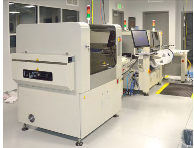
Figure 8: Campbell Company's fully automated SMT assembly line includes Manncorp's high-precision AP430 inline stencil printer, the three-head MC-389 pick and place system, and a CR-5000 convection reflow oven. With a full complement of component feeders and connecting conveyors, the line bore a price tag of nearly $250K, yet Campbell management believes it paid for itself in 12–18 months.
