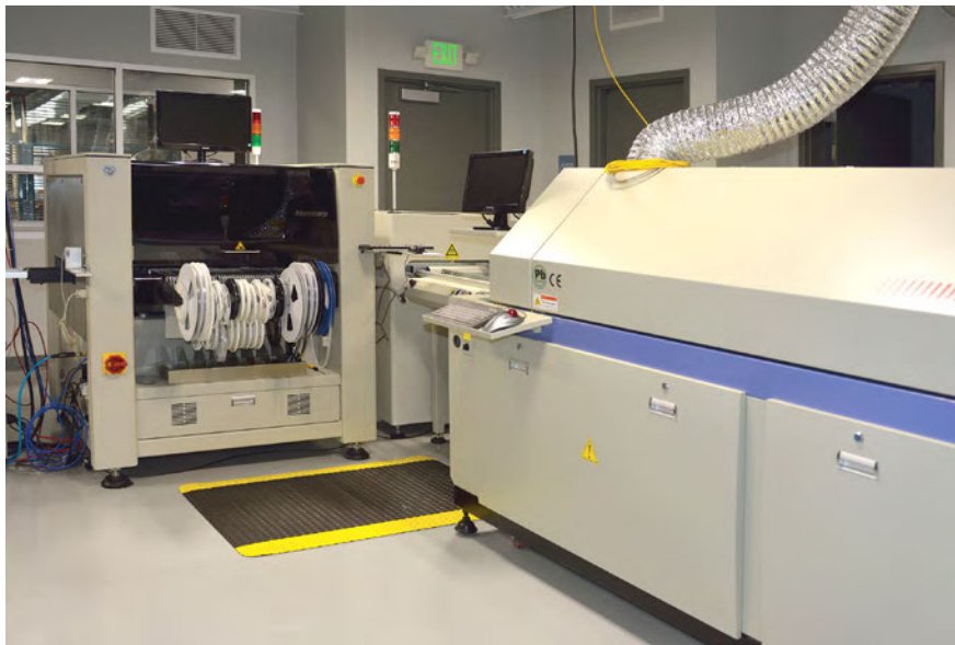
Figure 9: Due to space limitations, a 90° turning conveyor is positioned between Campbell Company's three-head MC-389 pick and place machine and their five-zone CR5000 convection reflow oven. Single-sourcing a complete turnkey SMT production line provides such benefits as seamless equipment integration, special package pricing, coordinated delivery, installation and training, and extended warranties.
